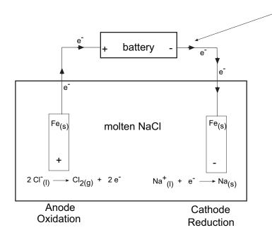
Chlorine gas is produced at the iron anode Solid sodium is deposited on the iron cathode
