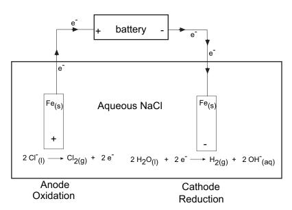
Chlorine gas is produced at the iron anode Hydrogen gas is produced at the iron cathode Teacher's Tools® Chemistry
