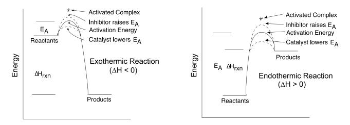
With the idea of activation energy, temperature really comes into play. The higher the temperature, the more energy that is in the system and the closer the molecules are to getting over the activation energy hump.
